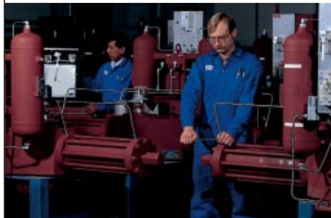
Gas/oil actuators undergoing final inspection before shipping
