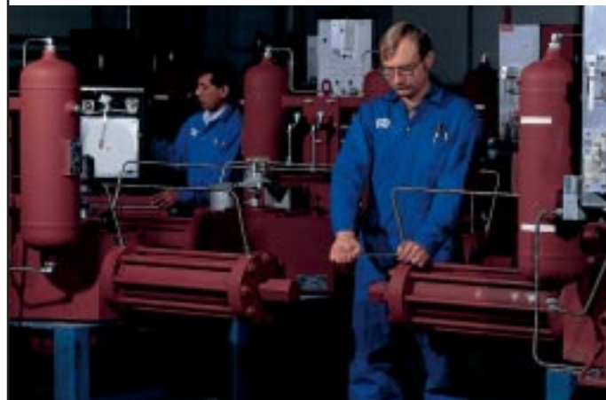
Gas/oil actuators undergoing final inspection before shipping
